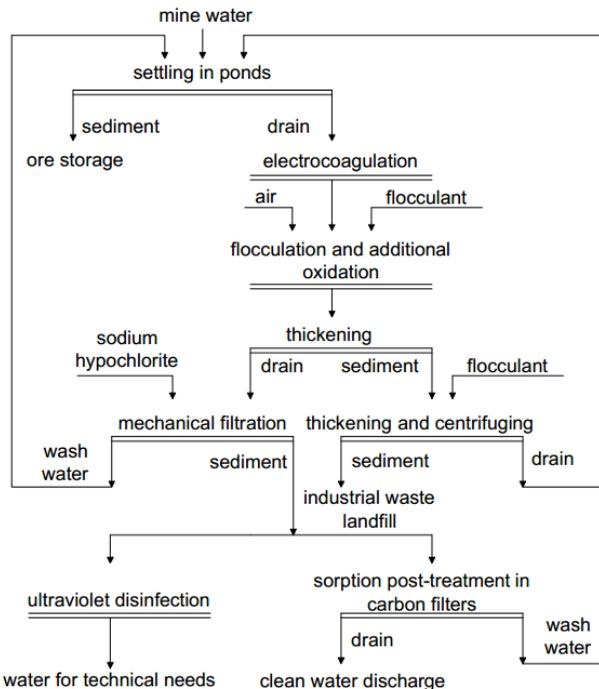
Figure Schematic diagram of mine water treatment
