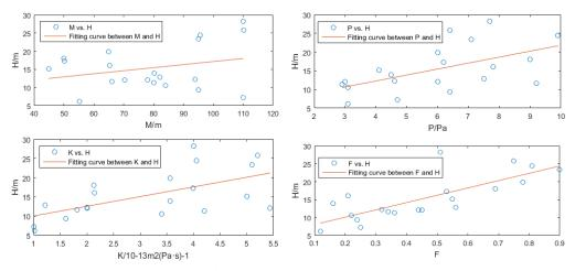
Figure 3 Fitting curve between the confined water rising zone and each influence index
