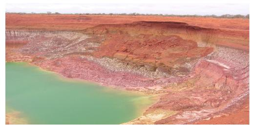
Photograph 1: Circular failure in saturated, extremely weathered Archaean rock
