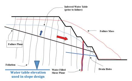
Figure 1: Diagrammatic section showing slope failure and groundwater assumptions
