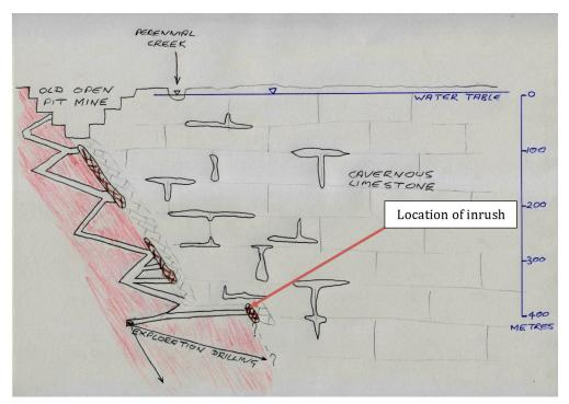
Figure 2: Diagrammatic location of the inrush to the underground mine
