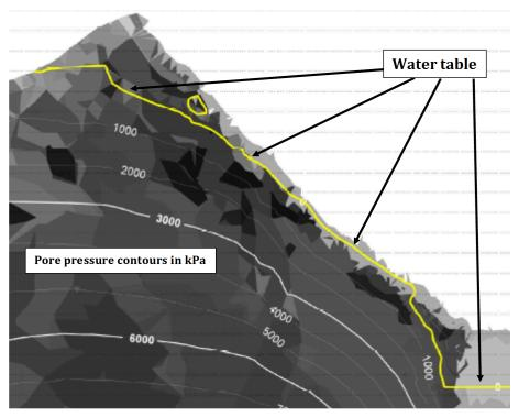
Figure 3: Example of pore pressure modelling in high relief terrain
