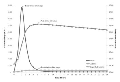
Figure 3 Discharge routing graph scheme in general.
