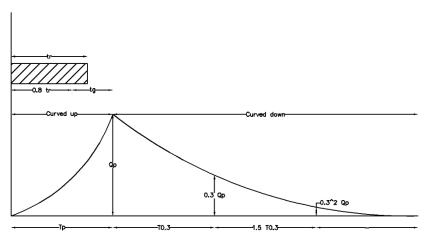
Figure 2 Hydrograph synthetic scheme of HSS Nakayasu.
