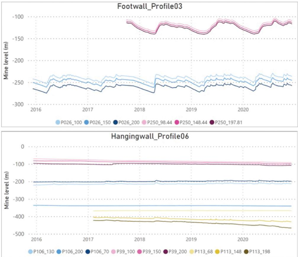
Figure 4 Comparative response of footwall and hangingwall VVPs to seasonal recharge.
