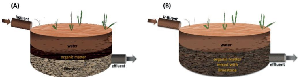
Figure 2 A typical diagrammatic representation of a RAPS setup (A) and a modified setup (B) currently used to treat mine water from the Witkranz discharge site.
