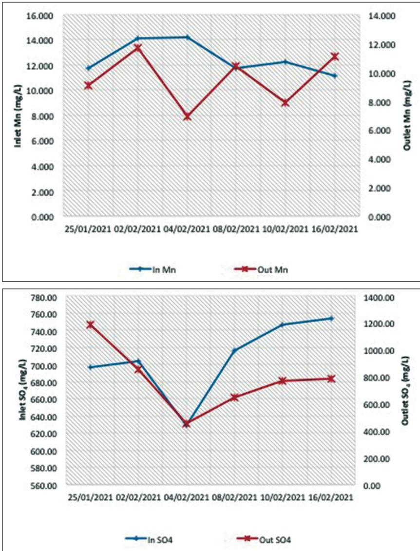
Figure 6 Graphs showing limited reduction of Mn (left) and SO<sub>4</sub> content (right) in RAPS 1.
