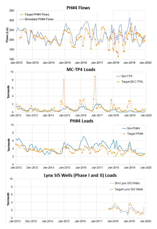
Figure 2 Simulated Monthly Flows to PH#4 and Zn Loads to Myra Creek, PH#4 and SIS wells 2012 to 2019.
