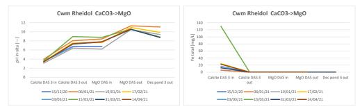
Figure 3 Evolution of pH (left) and total iron concentrations (right) along the Cwm Rheidol treatment train.
