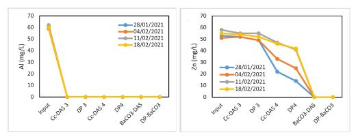
Figure 6 Evolution of total Al (left) and Zn concentrations (right) along the Parys Mountain laboratory columns.
