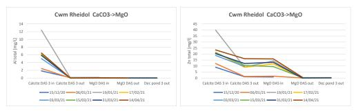
Figure 4 Evolution of total Al (left) and Zn concentrations (right) along the Cwm Rheidol treatment train.
