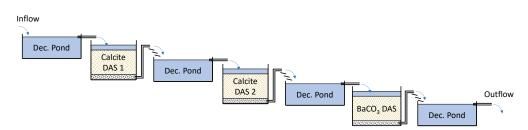
Figure 2 Schematic setup of the calcite-DAS + BaCO<sub>3</sub>-DAS laboratory columns for Parys Mountain.
