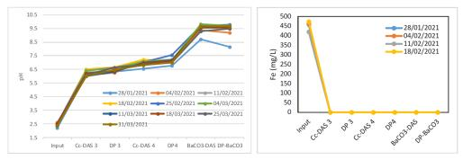
*Figure 5* Evolution of pH (left) and total iron concentrations (right) along the Parys Mountain laboratory columns.
