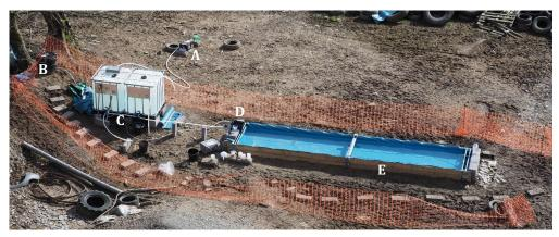
Figure 1 Arrangement of field trial at Abbey Consols. Adit standpipe (A), dosing solution tank (B), mine water IBCs (C), mixing tank (D) and settling pond (E).
