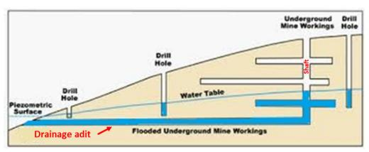
Figure 1. Schematic design of drainage adit (Source: adapted from Bourgeot et al., 2016).
