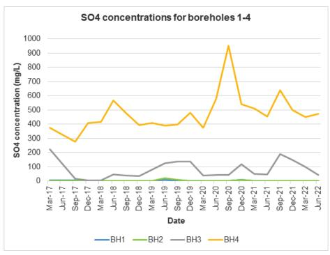
*Figure 2* Borehole sulfate concentrations since the commencement of irrigation. BH1 – deep upstream, BH2 – shallow upstream, BH3 – deep downstream, BH4 – shallow downstream
