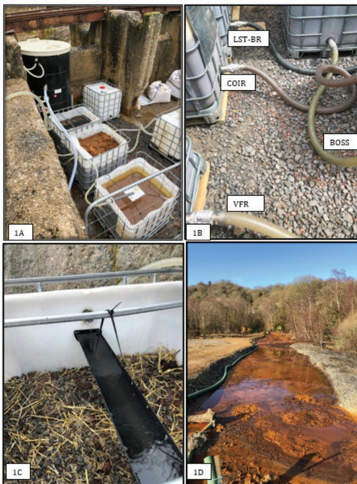
**Plate 1.** 1A: Cambokeels IBC trial. 1B: Cambokeels IBC effluent pipework. 1C: LST-BR substrate with gutter to distribute water. 1D: Bridford 'Iron Terraces'. (Images: Selina Bamforth).
