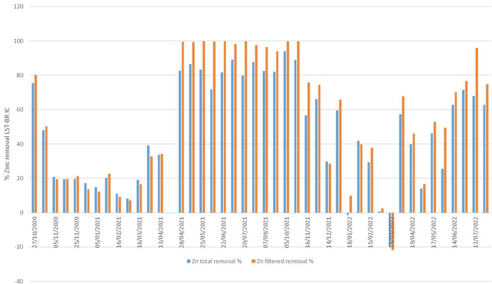
Figure 1B Cambokeels: zinc percentage removal in the LST-BR IBC (total and filtered (<0.45µm)).
