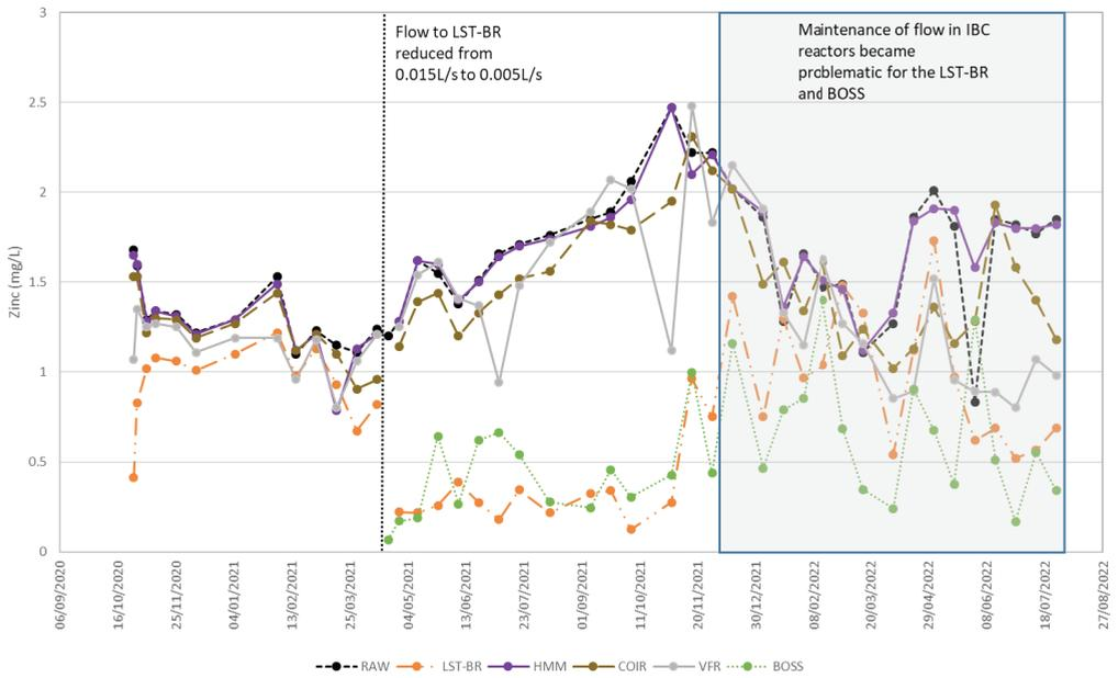
Figure 1A Cambokeels: zinc influent and effluents (see Table 1 for substrate descriptions).
