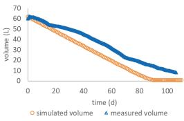
*Figure 1* Measured and simulated water mass evolution during lab scale test in the environmental chamber
