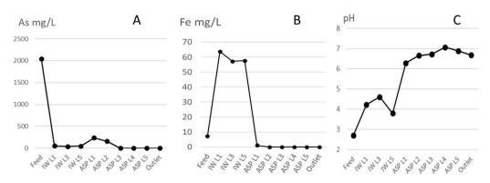
*Figure 5 Profiles of dissolved As (A), dissolved Fe (B) and pH (C) in the adsorption system composed of the columns working in series. IW column was fed with the seepage water. Ovive ASP commercial adsorbent (ASP), iron waste (IW). L1 to L5: sampling levels in the columns spaced 6 cm apart.*
