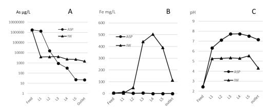
*Figure 4* Profiles of dissolved As (A), dissolved Fe (B) and pH (C) in the two adsorption columns independently fed with the seepage water on day 50. Ovive ASP commercial adsorbent (ASP), iron waste (IW). L1 to L5: sampling levels in the columns spaced 6 cm apart.
