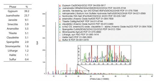
Figure 3 Results of XRD analysis of the final waste resulting from evaporation
