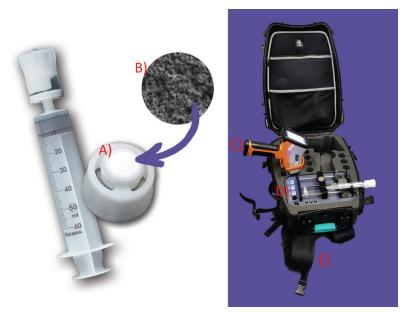
**Figure 1** 3AWater Multimetal Water Analysis System: A) metal collector made of a B) proprietary nanomaterial, C) handheld X-ray fluorescence (hXRF), D) Syringe pump and E) Accessory Kit backpack containing the everything needed for the analysis.
