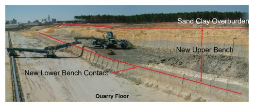
Figure 2 Quarry showing Benches and Bucket Wheel Excavator (Holcim US Inc ,2008)
