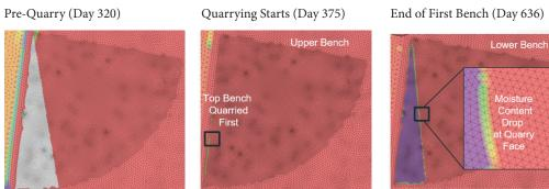
Figure 5 Simulation Results Showing Moisture Content in Walls
