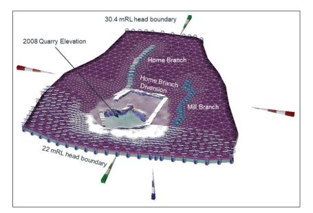
Figure 4 3D Numerical Model and Boundary Conditions
