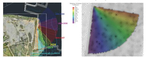
Figure 3 Example of Mine Sequencing in Feflow using User Defined Equations to form Nodal Distributions
