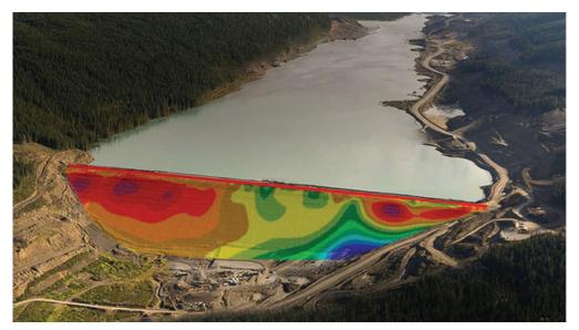
*Figure 4* Permanent resistivity array installation to reveal weak zones in a dam wall (https://www.lsi-lastem. com/products/G.Re.T.A./)
