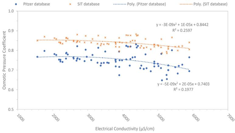
Figure 3 Plot of osmotic pressure coefficients calculated using the Pitzer and SIT databases versus EC for the feed
