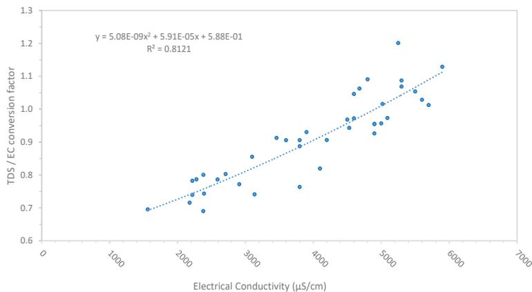
*Figure 1 Plot of TDS / EC conversion factor versus EC for the feed*
