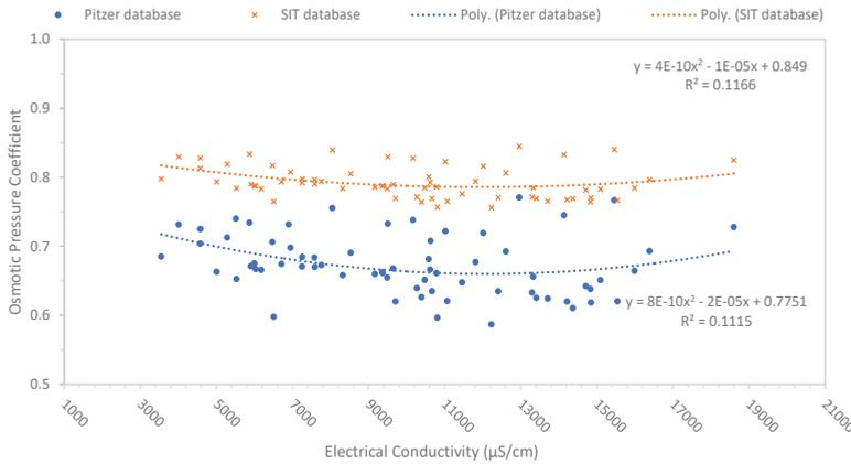
Figure 4 Plot of osmotic pressure coefficients calculated using the Pitzer and SIT databases versus EC for the concentrate
