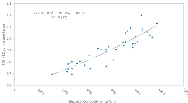
*Figure 2 Plot of TDS / EC conversion factor versus EC for the permeate*
