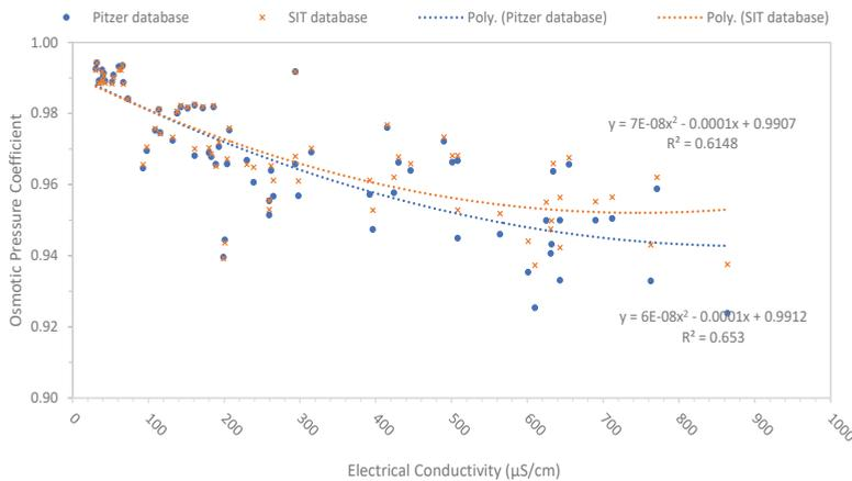
Figure 5 Plot of osmotic pressure coefficients calculated using the Pitzer and SIT databases versus EC for the permeate
