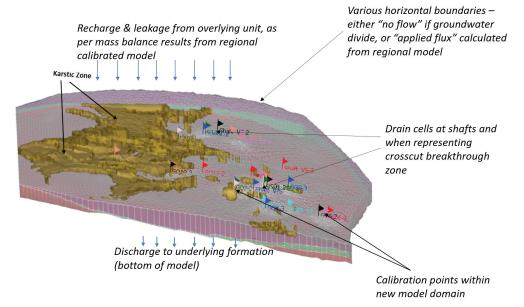
Figure 2 Example Boundary Conditions for Revised HGM Domain
