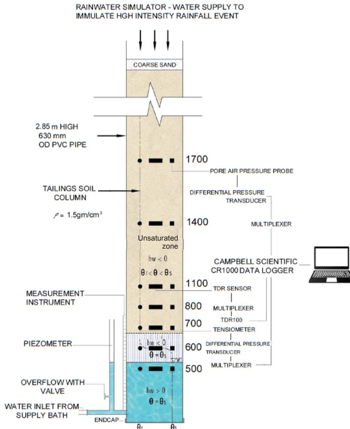
Figure 1 Schematic diagram of the column test apparatus and setup.  $\theta_r$  = residual soil water content,  $\theta_s$  = saturated soil water content.
