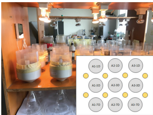
Figure 1 Schematic of Kinetic Test in the Laboratory using FDCLT method and Various Wet-Dry Cycle
