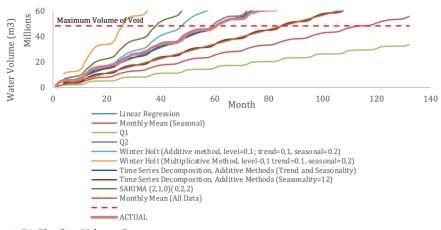
Figure 10 Pit Flooding Volume Curve
