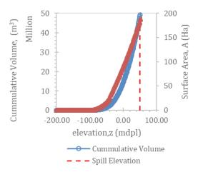
*Figure 3* Staging curve (elevation, surface area and volume) of void
