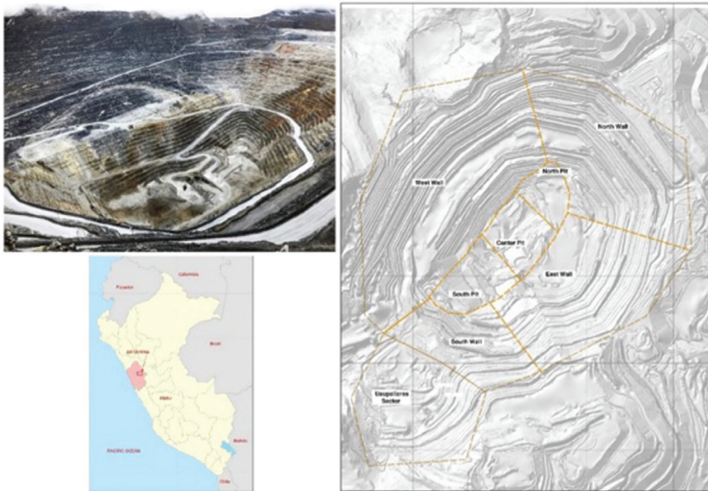
Figure 1 Location of Antamina mine in the Central Andes of Peru, Ancash Region, including an image of the pit layout, as well as the nomenclatures used to segregate behaviours for geological-geotechnical and hydrogeological management
