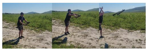
Figure 1 Hand launch of eBee X fixed-wing UAV
