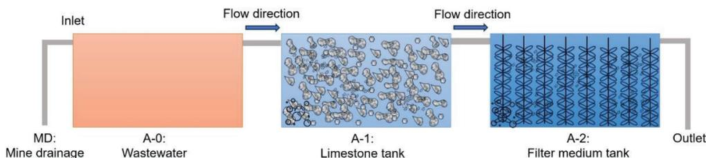
Figure 1 The schematic illustrates the design of the pilot-scale passive treatment system implemented within the underground tunnel of the legacy mine. The wastewater in A-0 was pumped from the mine drainage (MD) and discharged into A-1 before being directed A-2. Air agitators were installed in A-1 and A-2 to allow oxygen saturation in the treatment plant
