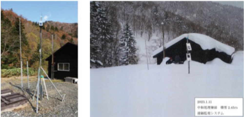
Figure 3 The transmitter and solar panel of Mine C (left; Summer, right; winter(2.45 m snow depth))
