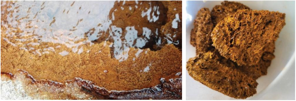
**Figure 1** Secondary mineral Schwertmannite; Left – formed in the mine water on the wall of the sedimentation basin; Right – detail with its porous structure.
