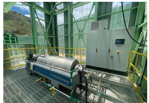
Figure 4 2-phase centrifuge processing neutralized waste sludge (Image: Jimmy Cordova).
