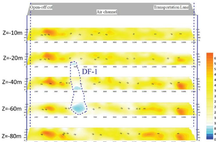
Figure 2 3D Electrical resistivity tomography (ERT) image of the 20223 working face floor.
