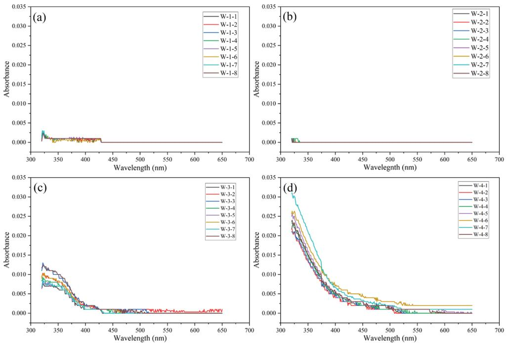
**Figure 3** Original spectral data of each aquifer. (a) 12-2~14-1 aquifer water samples, (b) 5 coal roof aquifer water samples, (c) quaternary aquifer water samples, (d) Ordovician limestone aquifer water samples.
