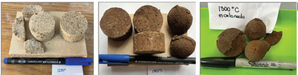
Figure 4 Specimens obtained at 1250 °C (a), 1300 °C linear (b) and 1300 °C staggered (c).
