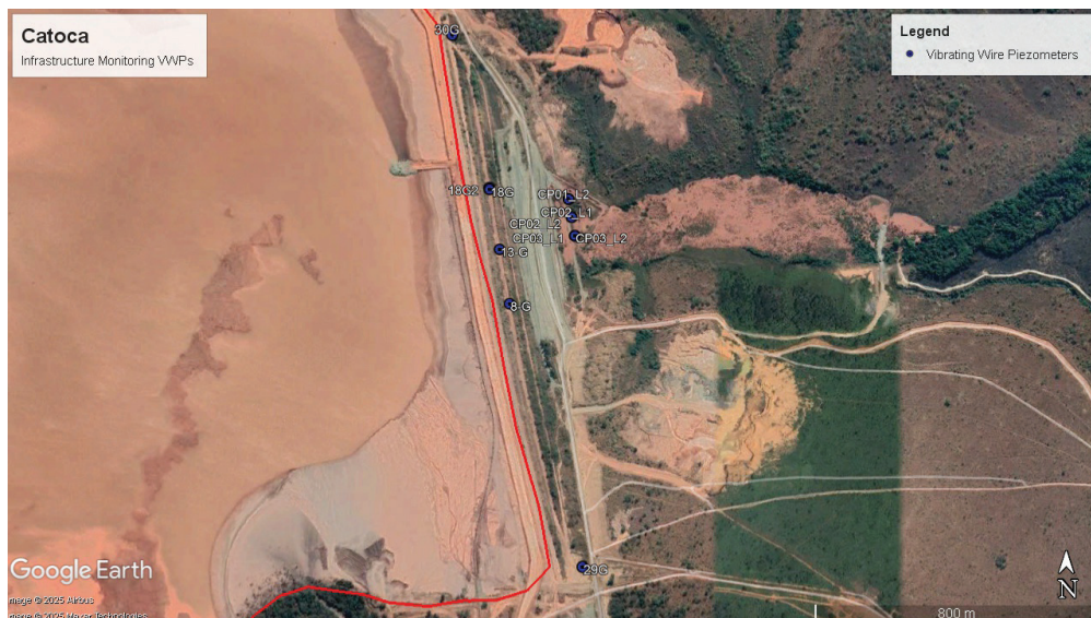
Figure 6 Locations of the monitoring VWPs in the active TSF.
