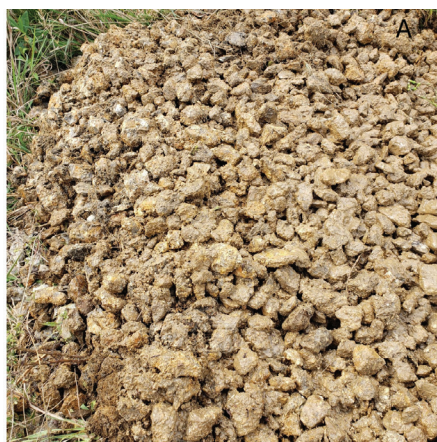
Figure 1 A) Aggregate fouled with AMD solids; B) aggregate after cleaning Both photos from the Kentucky Hollow oxalic limestone bed.
