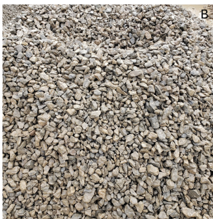
Figure 1 A) Aggregate fouled with AMD solids; B) aggregate after cleaning Both photos from the Kentucky Hollow oxalic limestone bed.
