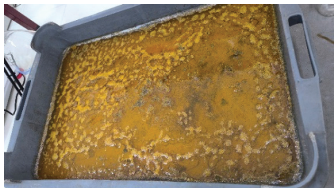
Figure 3 Lab-scale Pond with mine water from CMS and paper sludge. First precipitation of iron oxides.
