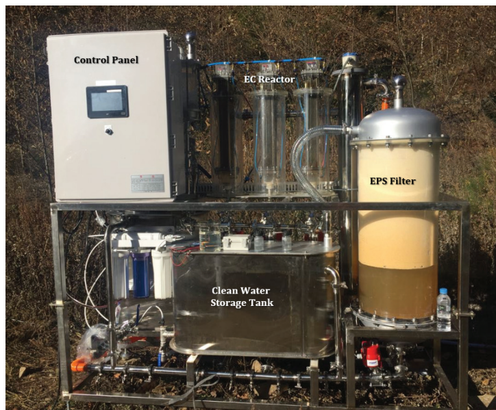
Figure 2 Field-scale electrocoagulation (EC) system installed at the Geumjeong Gold Mine.
